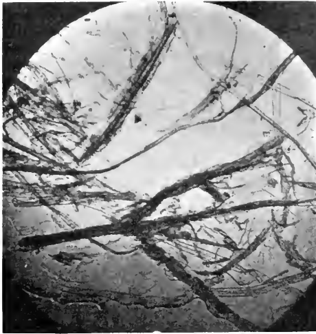
Mixture of 25 per cent sulphite and 75 per cent ground wood, by weight.
